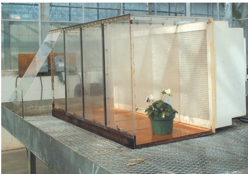
FIGURE 2. Negative Pressure Bench-top Containment Unit
